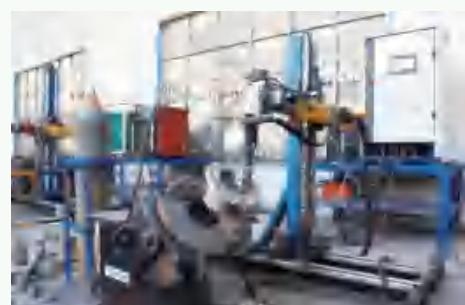
■ 管法兰自动焊 Pipe flange automatic welding
